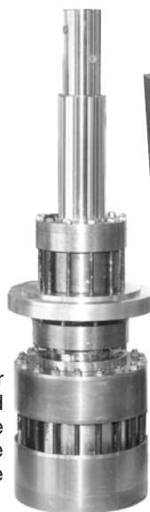
Special 2H Duplex Rotary Hydraulic Cylinder All Ports Located in Piston Rod 12 inch Bore x \frac{9}{16} inch Stroke 8 inch bore x 2 inch Stroke 1000 P.S.I. operating pressure
