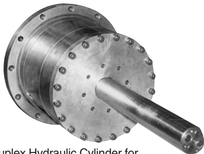
Duplex Hydraulic Cylinder for Hydraulic Rotating Chuck 8 inch Bore x 2 inch Stroke 12 \frac{1}{2} inch bore x \frac{9}{16} inch Stroke 1000 P.S.I. operating pressure
