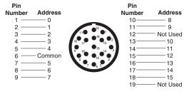
View into End Plate Connector - Male M23, 19-Pin
