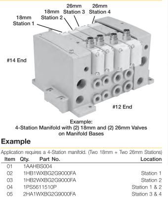
06 1PS5511510P Station 3 & 4 NOTE: Construct manifold assemblies from left to right while looking at the ports. Valves must be ordered as External Pilot when using Sandwich Regulator.
