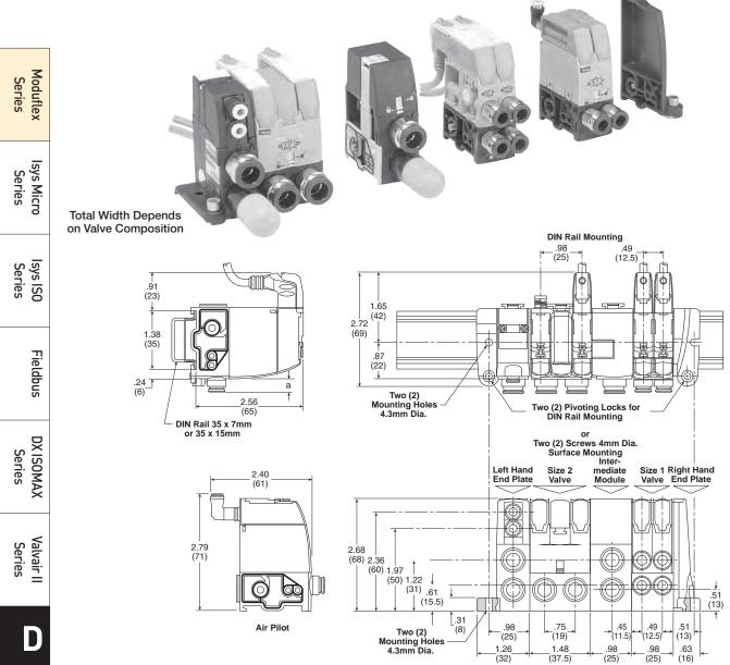
**Special Case:** 4/3 all ports blocked function within island version, add the dimensions of the dual P.O. check valve plugged into the island.
