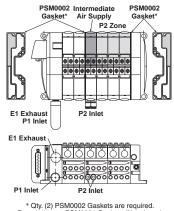
\* Qty. (2) PSM0002 Gaskets are required. Remainder are PSM0001 Gaskets (Not shown)
